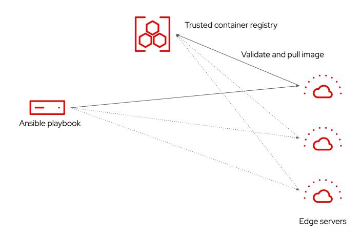
Ansible is used to orchestrate deployment of containers that are check for valid signing before being run
